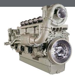
The 250MDA/MDB IMO II emissions compliant marine engine series includes both inline and V models and delivers a continuous power range from 1,498 bkW to 4,239 bkW (2,009 bhp to 5,685 bhp). The engines are based on a rugged one-piece iron casting mainframe for excellent vibration dampening characteristics and long-term stability to minimize bore distortion. Our easy to service unitized cylinder assembly concept enables quick change outs for increased engine uptime.
